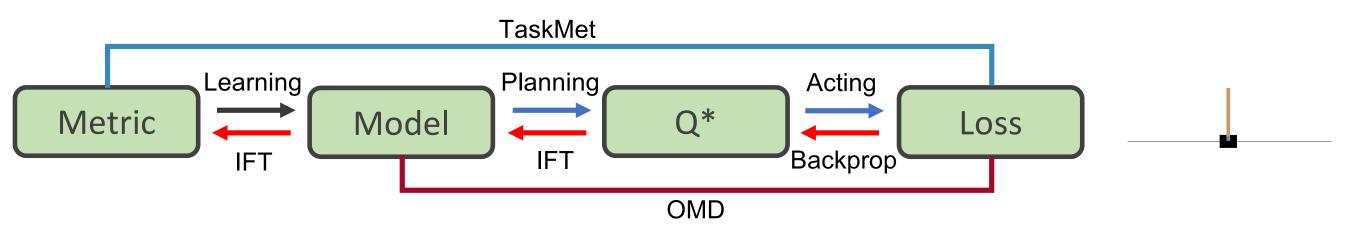
**Task:** find the optimal Q value function **Environment:** cartpole (#state dimensions: 4, #action dimensions: 2) Get the maximum return using trajectories from learned dynamics model **Experiment :** add noisy/distracting dimensions to the state space **Metric**  $\Lambda$ : diagonal and not conditioned on x**Result: t**he learned metric downweights the noisy dimensions, allowing the prediction model to use its capacity on task relevant features only
